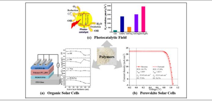
Figure 1: Applications of polymers in energy conversion and storage field.
