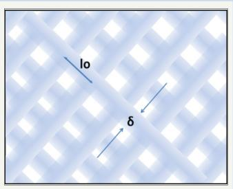
**Figure 3:** The appearance of two characteristic scales in structured body, the distance between slide lines and -the thickness of plastic zone, the integer n is equal to 25.
