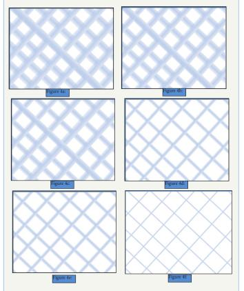
**Figures 4 (a-f):** Illustrate the successive increasing of elastic area (white color) of a body with simplest common stress and the concentration of plastic zones near sliding lines. The integer n is equal from 30 up to 100.
