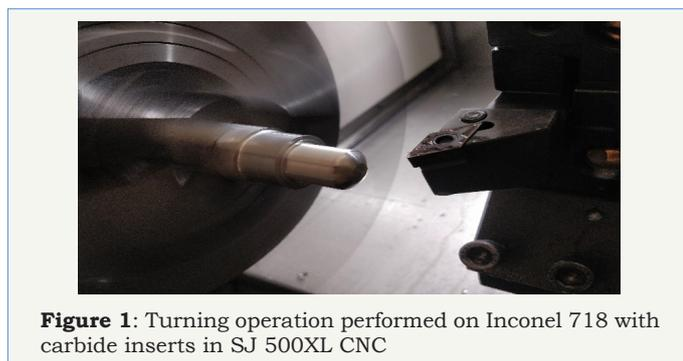
**Figure 1:** Turning operation performed on Inconel 718 with carbide inserts in SJ 500XL CNC
