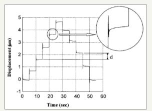
**Figure 3:** Step response of the piezoelectric actuator with displacement difference resulted from the hysteresis [34].
