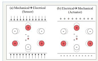
**Figure 1:** Sensing and actuating abilities from piezoelectric effect [10].
