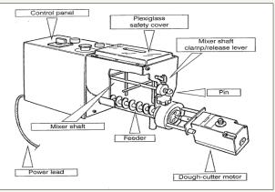
Figure 1: Schematic view of Dolly pasta machine.
