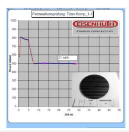
**Figure 3:** Titanium composite plate: The curve from approx. 10 seconds is horizontal.
