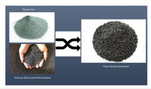
**Figure 1:** Mixture of polymers and titanium powder to titanium composite material.
