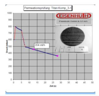
**Figure 5:** Titanium composite plate: The curve from approx. 10 seconds onwards drops very slightly.
