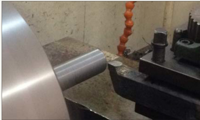
Figure 5: Machining tests using the samples as cutting tools to measure the performance.
