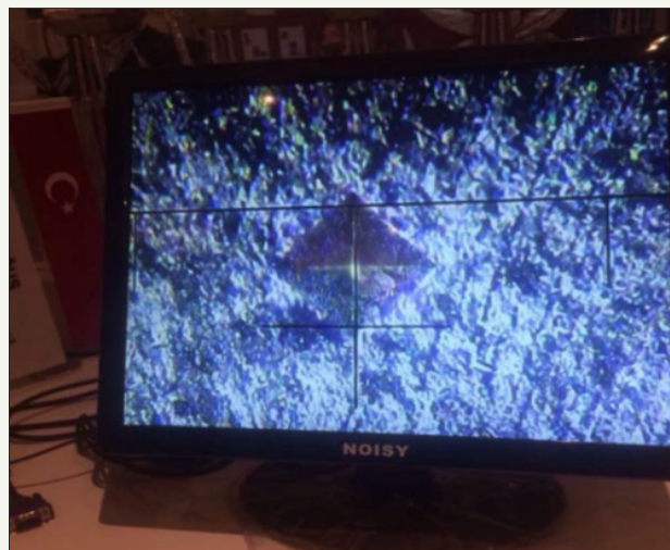
Figure 4: Vickers microhardness measurements.
