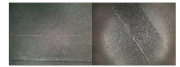
**Figure 3:** Microscopy pictures of the surfaces of sample 1 (left) and 3 (right) after the mechanical roughness measurement.
